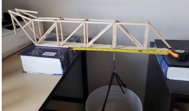
Figure 8: load bridge setup
