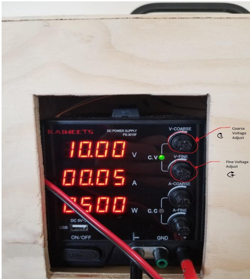
Figure 02 Power Supply Adjustment
