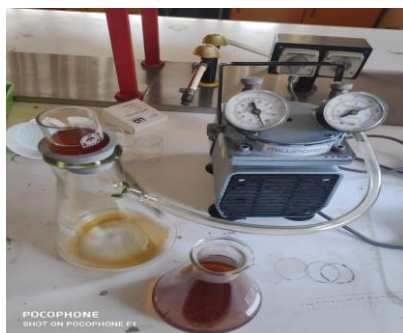
Figure 3 9 - Filtration process through suction during total fibre determination
