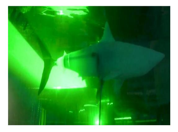
Figure 11: The Shortfin Mako model positioned in the flume with the laser illuminating the streamwise-spanwise (x, y) plane behind the fork of the lunate caudal fin.
