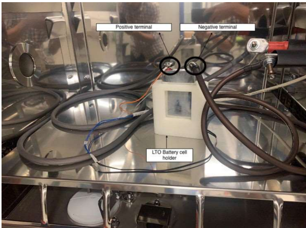
Figure 12 Experimental set-up of LTO battery in WEISS Technik Weather chamber
