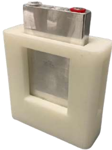
Figure 10 3D printed battery cell holder
