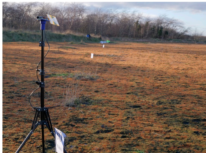
Figure 5. Setup for the received signal strength indicator (RSSI) tests for receive and transmit antennas.
