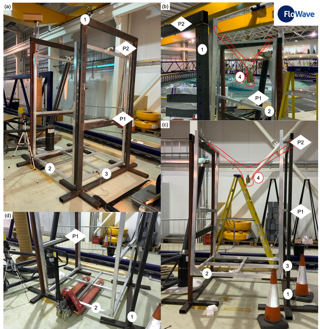
Figure 1. Overview of the swing with support structure (1), swing (2), inclinometer (3) and masses including the rope highlighted with a red line (4) as well as the two different pivot axis (P1 and P2): (a) Balanced swing at the pivot axis P1. (b,c) Swing at the pivot axis P2 with full calibration weights (d) Support structure moved to remove the swing.
