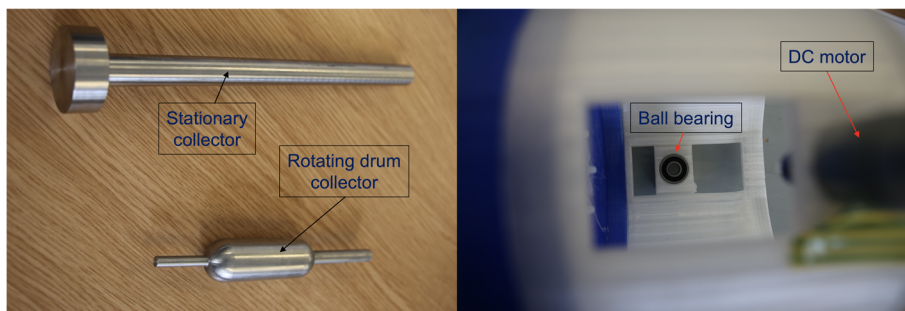
Fig. 7 Left: Photograph of the stainless steel stationary flat collector (top) and the rotating drum collector (bottom). Right: Photograph of the ball bearing, which houses the shaft of the rotating drum collector. The blurry part on the right side is the DC motor
