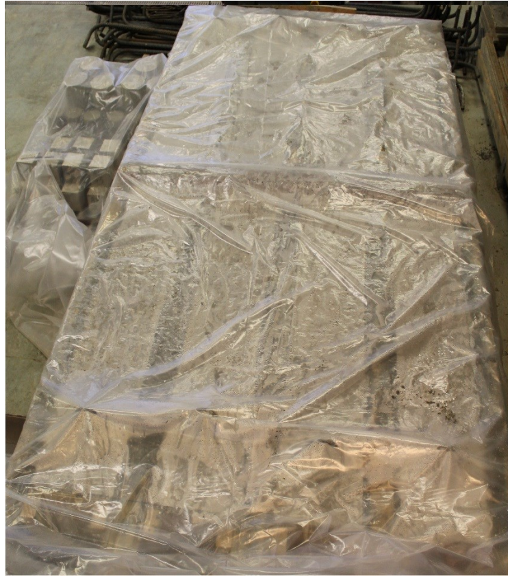
Figure 3.9: Beams and air cured specimens wrapped for curing
