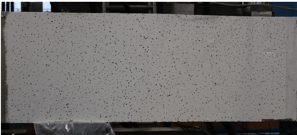
Figure 3.15: Typical speckle pattern for DIC
