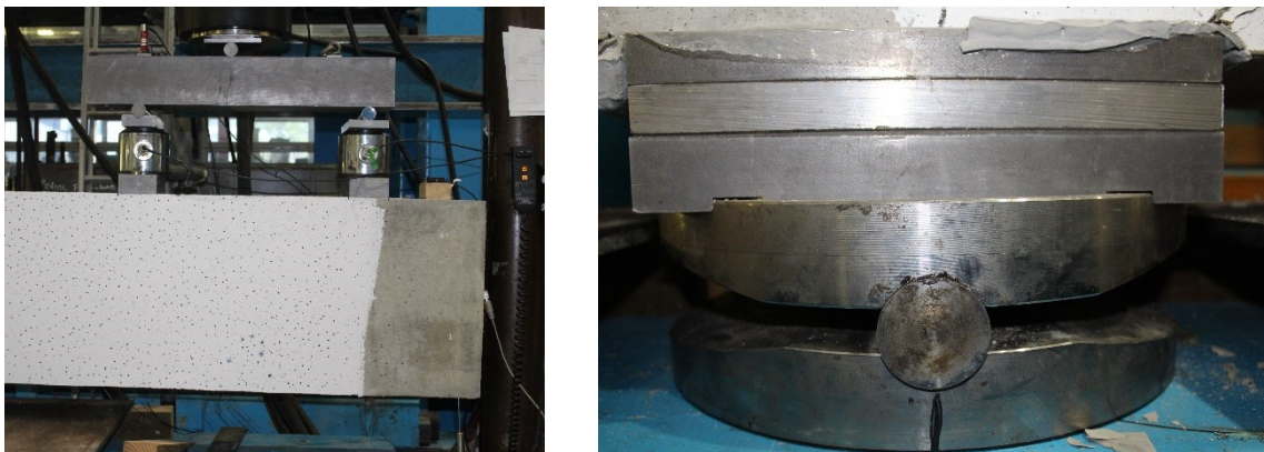
Figure 3.11: Load cells (Left) and Seating ball (Right) in series A of beams
