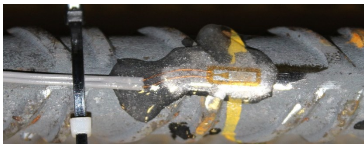
Figure 3.22: Fixing and coating of a strain gauge
