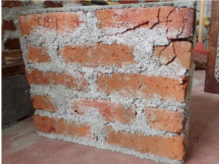
Figure 11. Brickwork prism failure in compression tests
