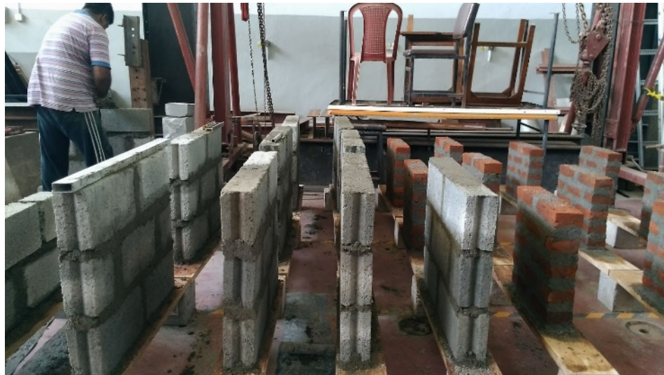
Figure 9. Masonry prism construction
