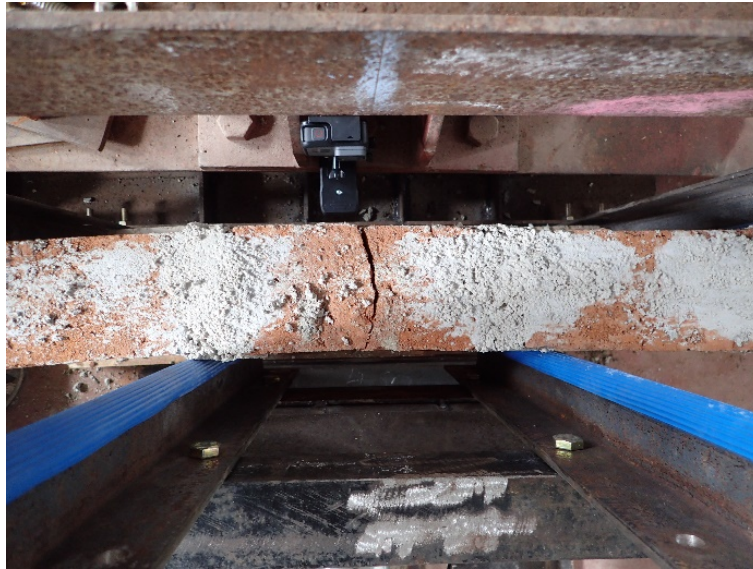
Figure 13. Perpendicular to bed joint flexural test failure
