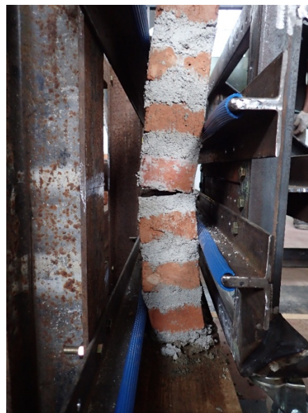
373 Figure 12. Parallel bed joint flexural test failure
