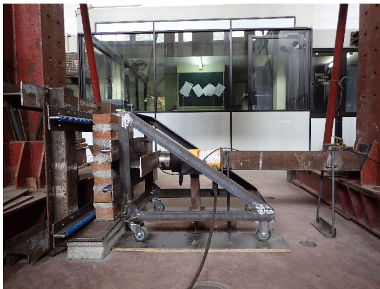
Figure 10. Parallel to bed joint flexural test
