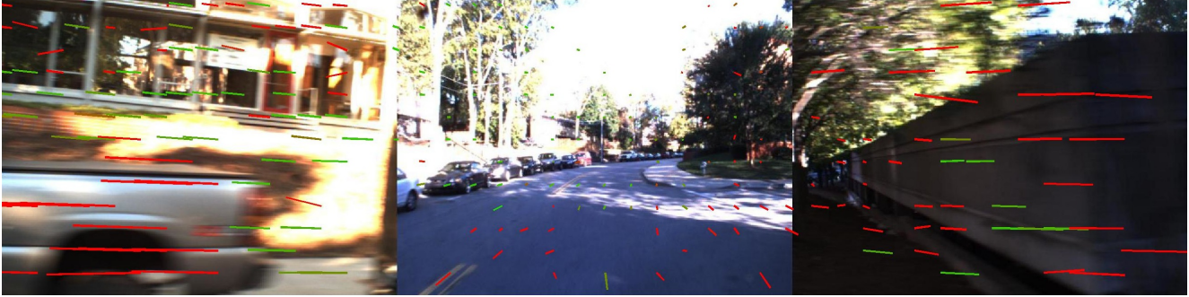
Figure 7: Detection of outliers in the sparse optical flow in a frame from the 3-camera outdoor driving sequence. Colored lines are sparse optical flow, ranging from green when p(\text{inlier}) = 1 , to red when p(\text{inlier}) = 0 . Sparse flow vectors that are inconsistent with the linear flow subspace have low inlier probability. Vectors on the moving pickup truck, in the textureless regions of the road, and on the very close and very far structure of the wall are labelled as outliers.
