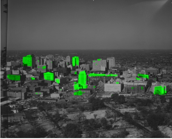
Figure 3: Object Observations. Our framework reasons about observations of 3D objects in images. We group the 3D points from SfM into larger structures and count the detection of at least one point in the group as an observation of the entire structure. Regions highlighted in green (above) represent observed objects in this image. False negative observations are undesirable but unavoidable, and we account for them in our probabilistic framework.
