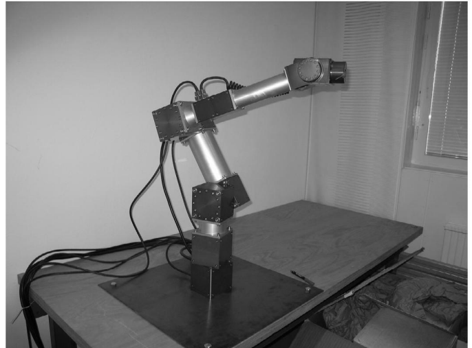
Fig. 1 The manipulator used for teleoperation studies
