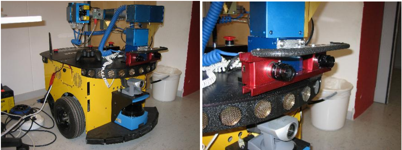
Fig. 1. Left: The experimental platform, the PowerBot Dumbo from ActivMedia. Right: A close up of the Videre stereo rig used in the experiments.
