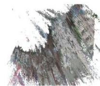
Figure 3. Lateral view of the point cloud obtained from 91 frames, with clearly visible distortions.
