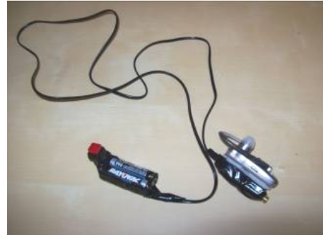
Figure 5. Ear-mounted laser pointer and a wired button
