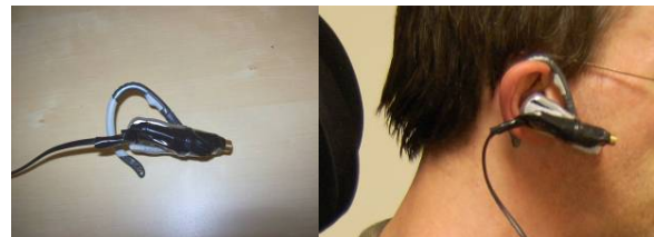
Figure 6. Ear-mounted laser pointer worn by a participant
