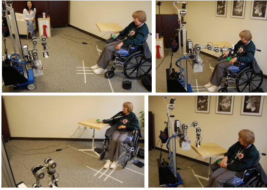
Fig. 8. Top: The user shines the laser point onto her lap, the robot delivers the object to user (direct delivery). Bottom: The user shines the laser point onto the table, the robot delivers the object to the table (indirect delivery).
