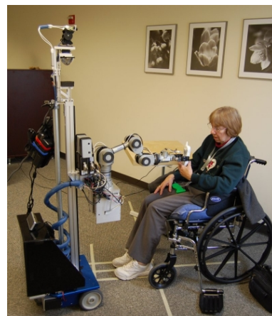
Fig. 1. EL-E handing a cordless phone to an ALS patient. Photos used with patient permission and IRB approval.
