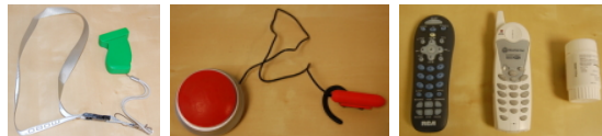
Fig. 7. Left: Hand-held laser pointer. Middle: Ear-mounted laser pointer. Right: The three objects used in this study - TV remote, cordless phone and medicine bottle.
