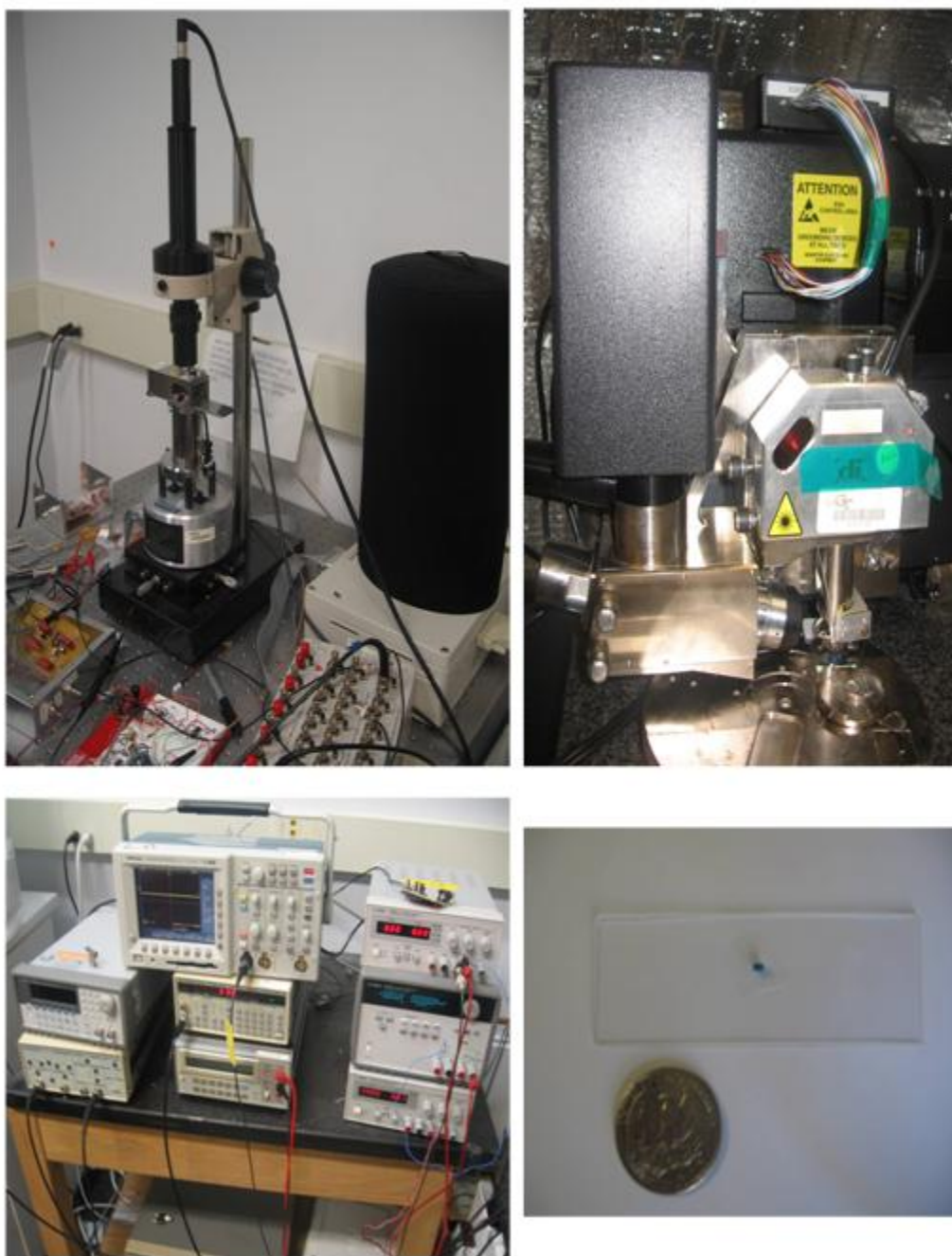
Figure 7.12: Atomic force microscopes (top) used for imaging local micro/nano scale viscoelastic properties of seal surfaces. Also shown is the cantilever driving and data acquisition circuit (bottom left) and a seal sample used (bottom right). (AFM setup from the lab of Prof. Levent Degertekin at Georgia Tech.)
