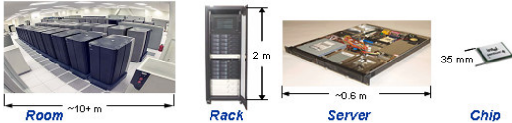
Figure 1.1. Data center and its multi-scale nature
