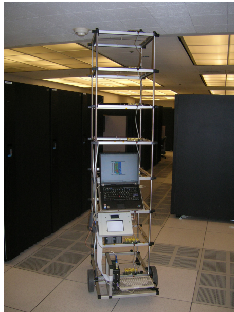
Figure 8.2. Mobile Measurement Technology (MMT): 3D temperature mapping tool (courtesy of Dr. Hendrik Hamann)
