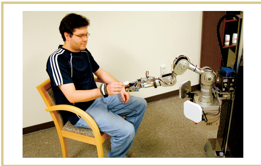
Figure 4. EL-E delivers a tagged medication bottle to a person wearing a tagged wristband. Tagging people and objects facilitates human-robot interaction and provides identities with high confidence, which is crucial for applications like delivering medicine.
