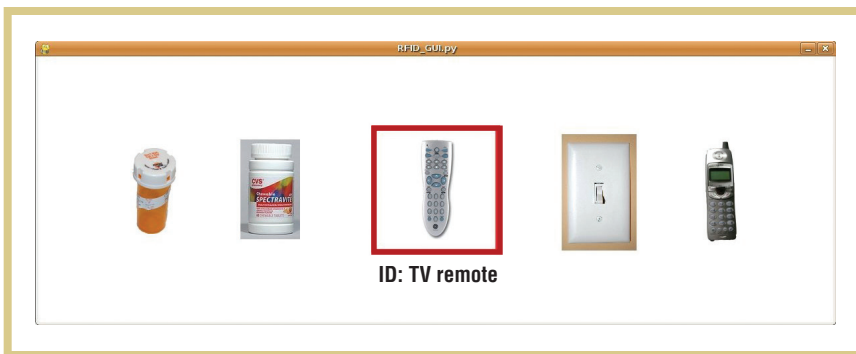
Figure 2. EL-E's user interface (UI). On the basis of RFID-tagged objects it senses nearby, EL-E generates a context-aware remote UI on-the-fly. From this UI, users select an object and action for the robot to perform.
