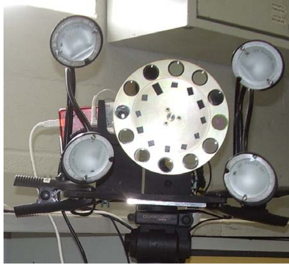
Figure 1: The spectral imaging system. The filter wheel and illumination are visible. The camera is located behind the left side of the filter wheel.
