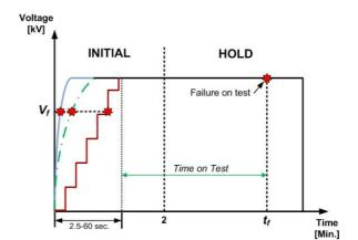
Figure 1: Withstand Test "Initial" and "Hold" Phases
