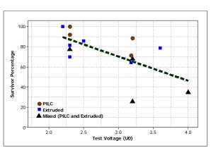
Figure 4: Percentage of Surviving Segments Versus Test Voltage (U<sub>0</sub>)
