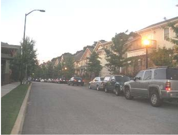
Figure 3.2-9: Parallel parking and a green buffer protect the sidewalk from street traffic.
