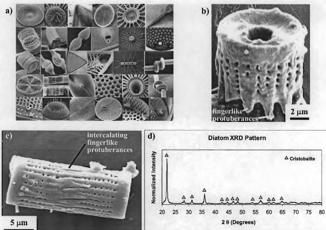
Figure 1. a) SE images of SiO<sub>2</sub>-based microshells (frustules) associated with 30 diatom species (assembled by M. Hildebrand, Univ. California at San Diego, from images in [1]); b), c) SE images of *Aulacoseira* frustules (obtained as flame-polished diatomaceous earth powder from a local vendor); d) XRD pattern obtained from *Aulacoseira* diatom frustules.
