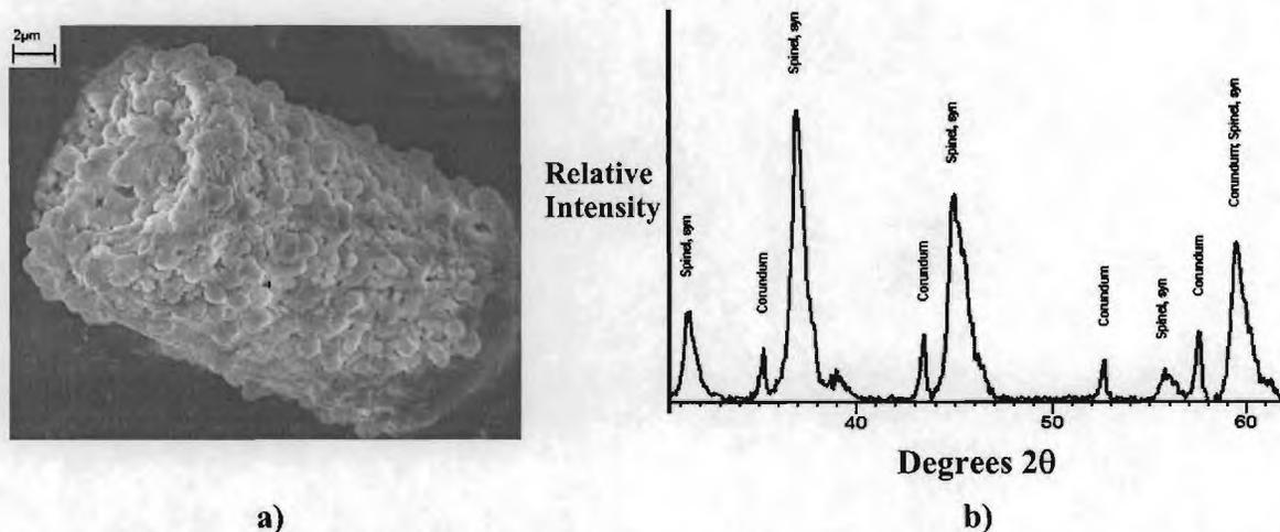
Figure 4. a) A SE image and b) an XRD pattern obtained after applying a sol-gel-derived alumina coating on magnesia frustule replicas, firing at  $1100^\circ\text{C}$ , and then selectively dissolving the underlying magnesia away.
