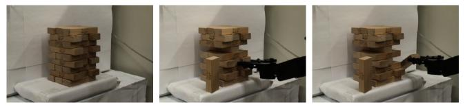
(a) Full tower setup with eight side blocks pulled (b) A new block is selected by the Block Removal (c) The block is successfully extracted from the 0.5cm forward. Planner. tower.
