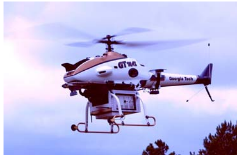
Figure 6 – GTMax Research UAV
