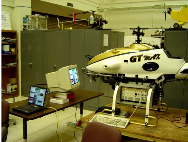
Fig. 13. Simulated and recorded-actual images presented to the image processing and mission management subsystems in laboratory testing (camera under nose of helicopter has lower right of white computer monitor in view)
