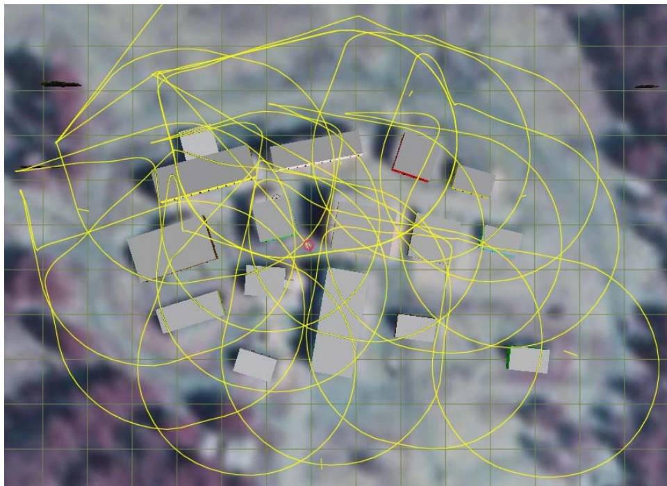
Fig. 15. Ground track during mission attempt, start is coming in from the top, finish at circle near center of image. The building with symbol is top center, and is circled twice.
