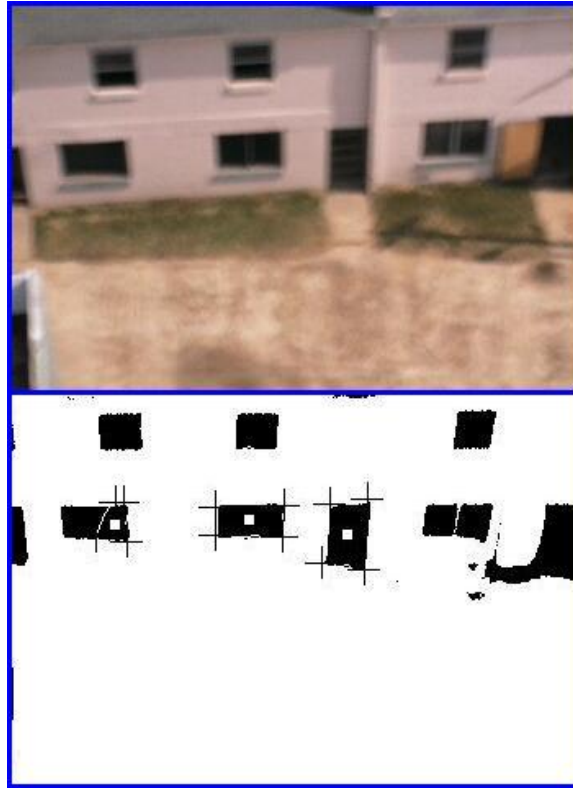
Fig. 9. Identification of the geometric characteristics of the contours.
