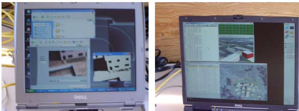
Fig. 5 Ground Control Station displays, (left) real-time video from the onboard camera and processed imagery; (right) monitoring onboard systems with a moving-map display, and other monitoring tools
