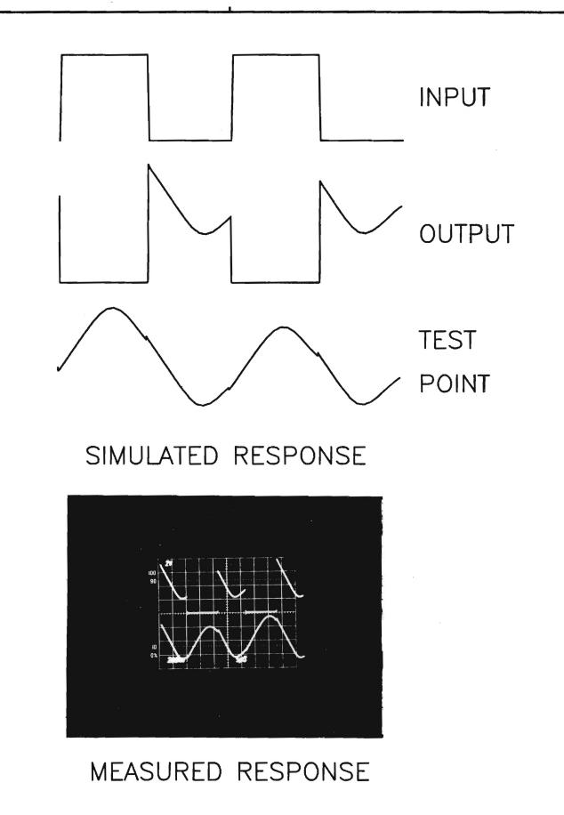
FIGURE 2. COMPARISON OF MEASURED AND CALCULATED RESPONSES TO 10 MICROSECOND PULSE.
