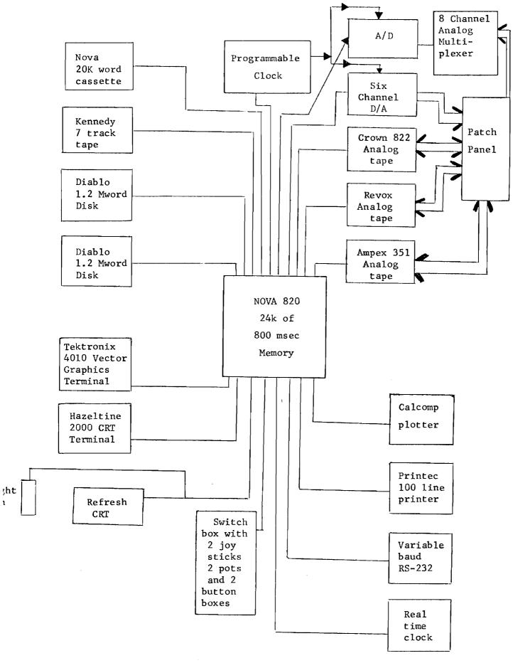
Figure 1. Layout of NOVA 820 Facility used in the Speech Algorithm Development and Testing
