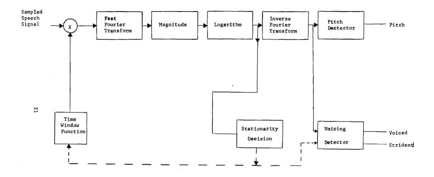
Figure 6. A Block Diagram of the Proposed Adaptive Cepstrum Pitch Detector
