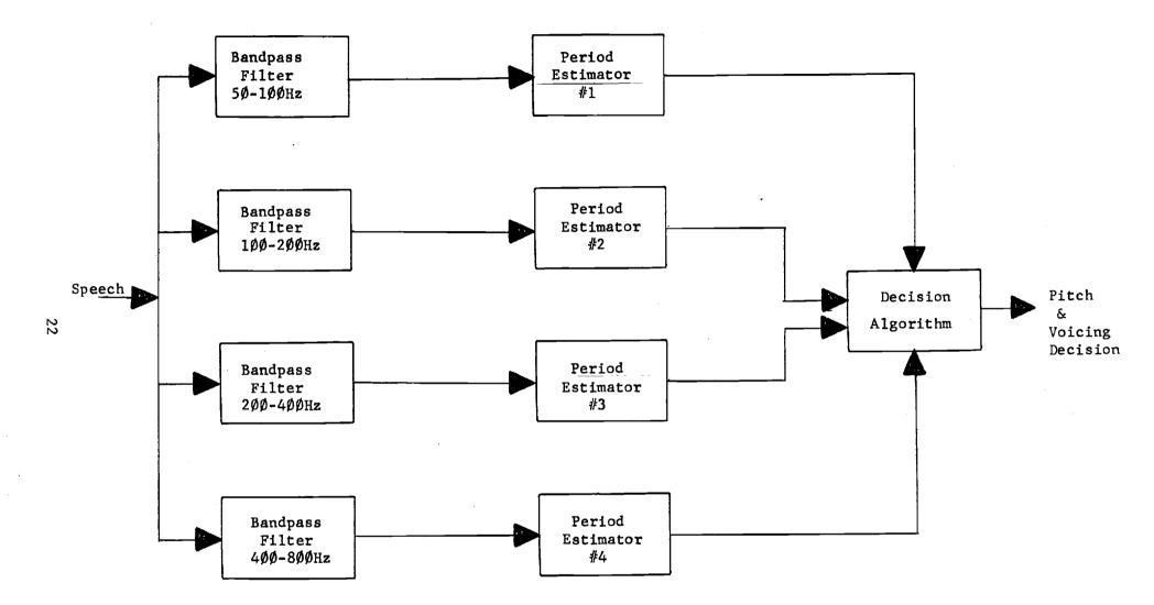
Figure 7. Multi-Band Pitch Detector
