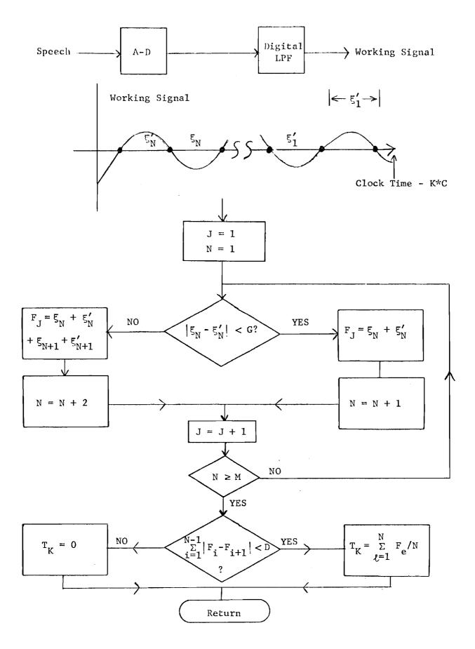
Figure 3. Zero Crossing Pitch Detector
