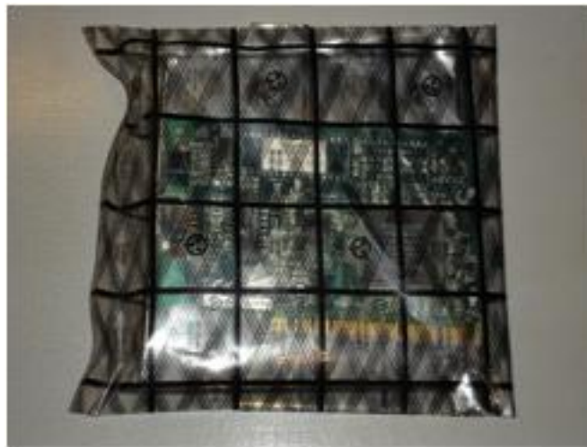
Figure 1.4 Example of a carbon black polymer-composite being used to provide electrostatic shielding in the packaging of electronics components that are sensitive to electrostatic discharge. [41]
