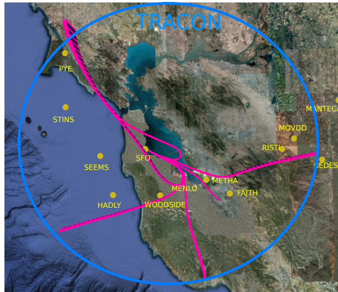
Figure 48: Centroids of the clusters and reporting points/way-points for SFO arrivals. Those centroids differ from the ones in Figure 61 because the algorithm was run with different parameters with a smaller sensitivity.
