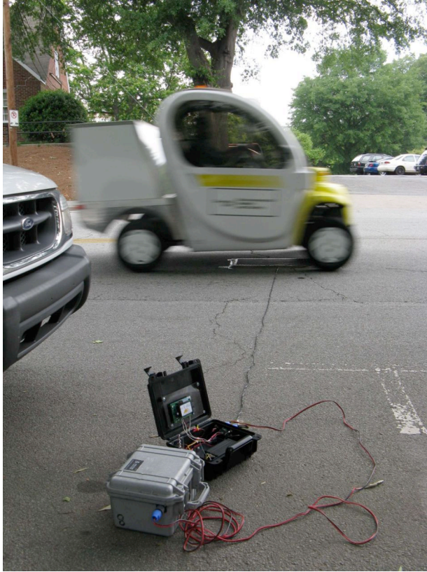
Figure 34 - DSP-15 Detecting A Georgia Tech "Golf Cart" (Fifth Field Test)
