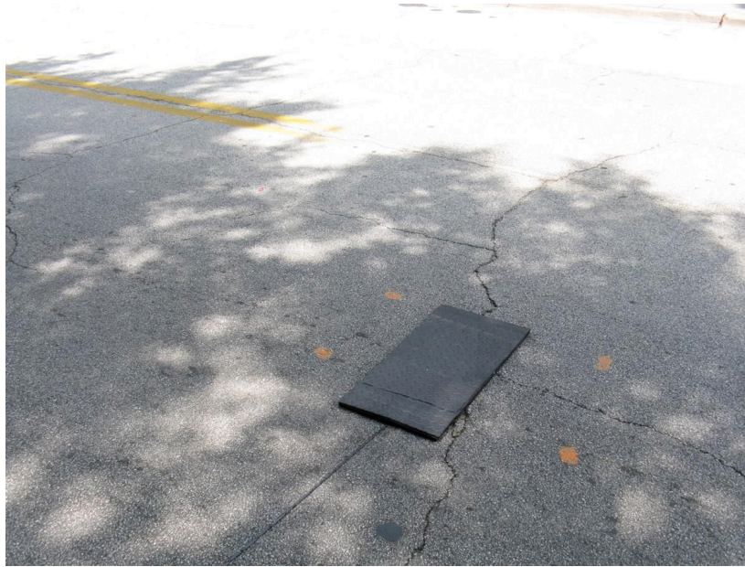
Figure 43 - Intermediate Size Loop Deployed Longitudinally, During Seventh Field Test
