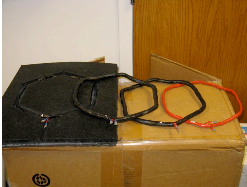
Figure 36 - Small Detector Pad With Four Hexagonal Loops (10" Diameter). From Left: 6 Turns, 12 Turns, 29 Turns, and 88 Turns of Wire
