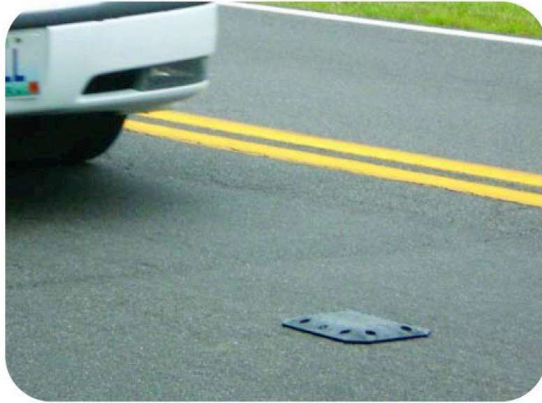
Figure 3 - Hi-Star® Traffic Counter Affixed to Pavement in Rubber Housing [8]
