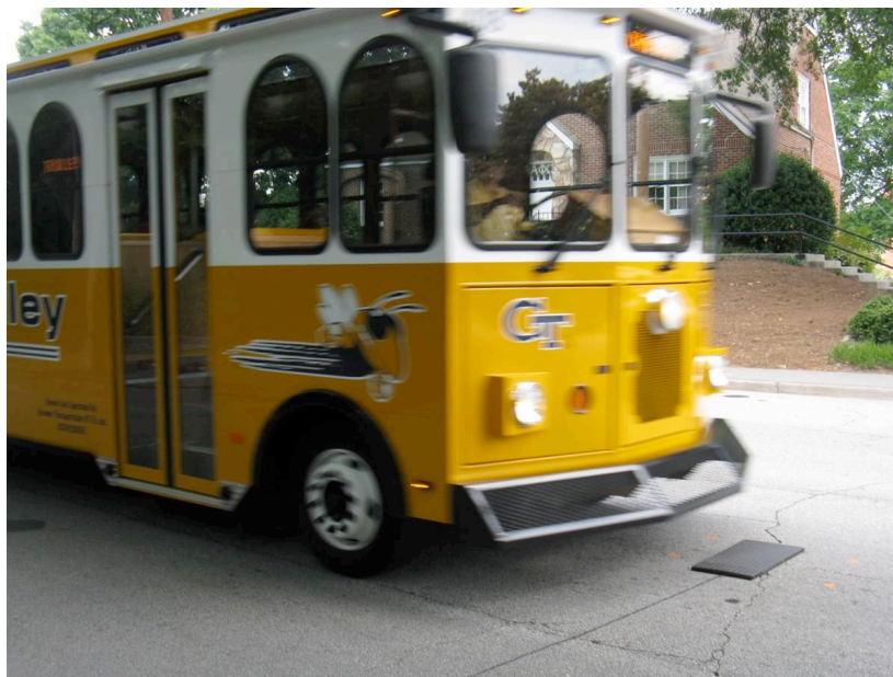
Figure 44 - "Tech Trolley" Driving Over Intermediate-Sized Loop Mounted Traverse (Seventh Field Test)
