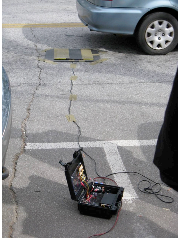
Figure 22 – First Field Test, 2/13/09, Showing RSN1000 and Detector in Enclosure
