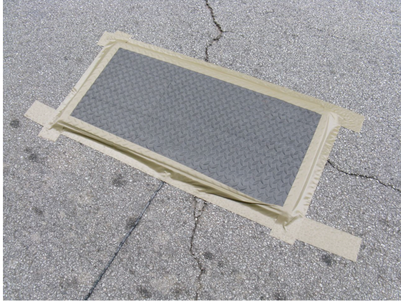
Figure 32 - Detector Pad Affixed to Pavement (Fifth Field Test)
