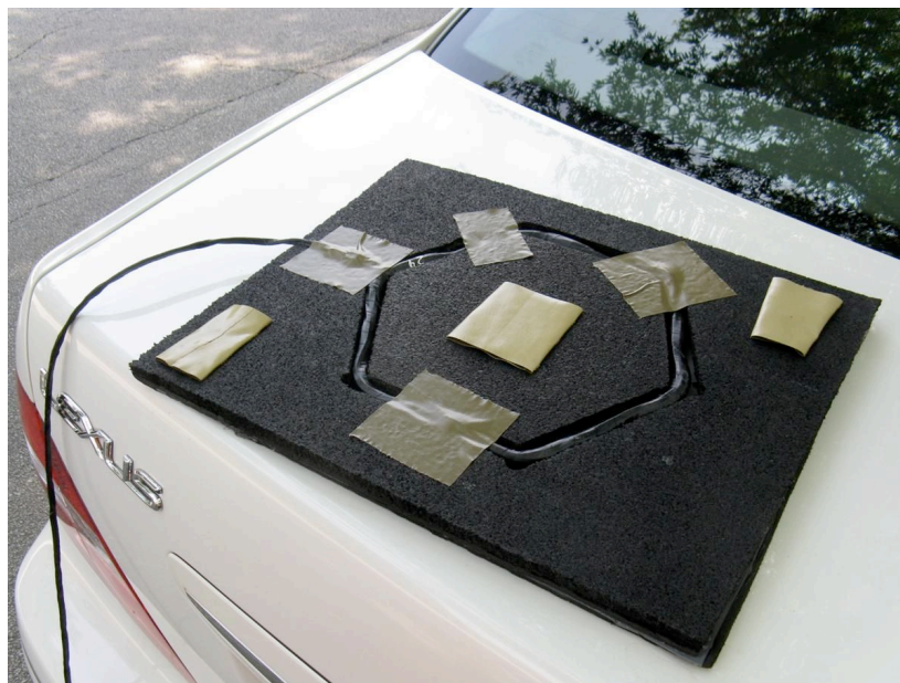
Figure 38 - Detector Pad with 12-Turn Loop. Looped Tape is Applied to Affix Pad to Pavement (Sixth Field Test)
