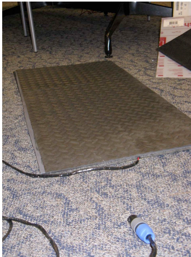
Figure 18 – Second Generation Loop Assembly Made of Recycled Tire, and Close-up of Electrical Interconnect
