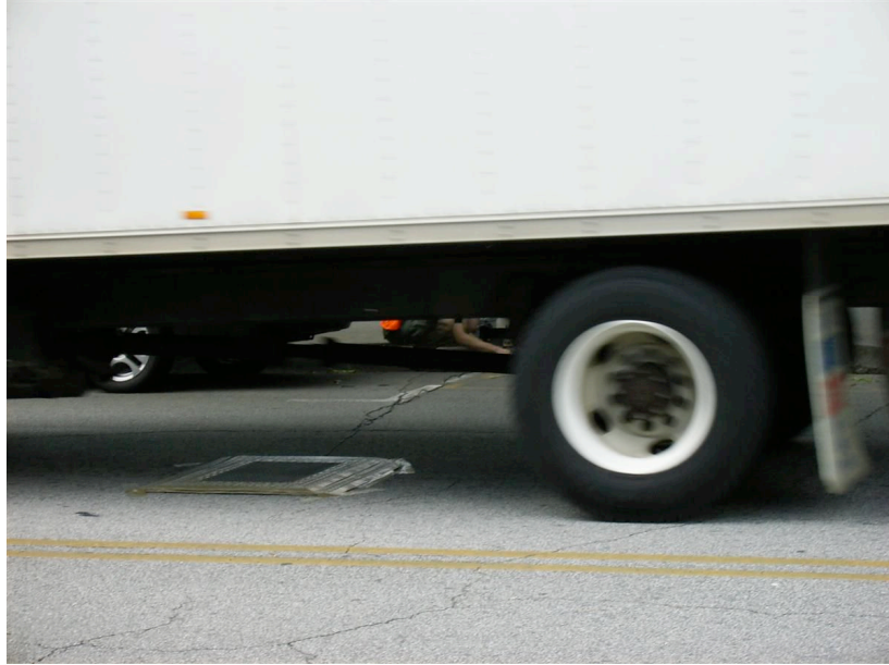
Figure 27 - Loop Assembly Detecting an 18-Wheeler (Third Field Test)
