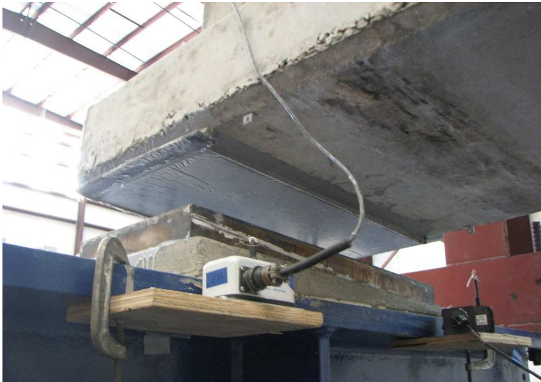
Figure 4.16 – High-modulus epoxy leveling retrofit
