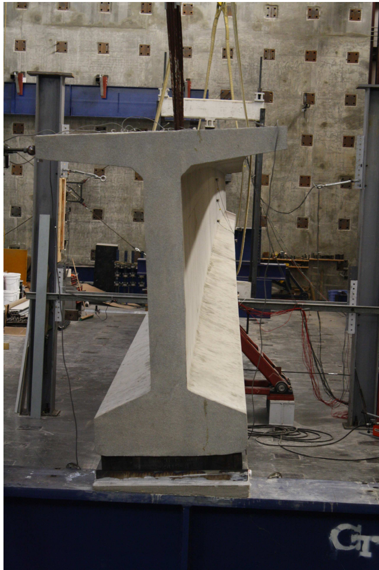
Figure E.5 – BT-54 end view showing initial rotation
