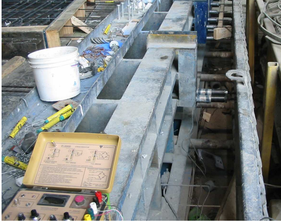
Figure 2.4 – Measurement of prestressing strand force
