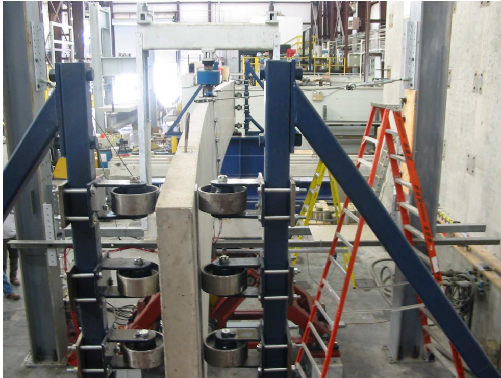
Figure 5.19 – End view of sweep and rotation for loading #3 of Beam B2A
