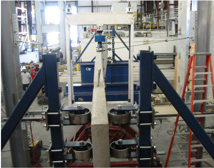
Figure 5.45 –End view of Beam B1B in buckled position
