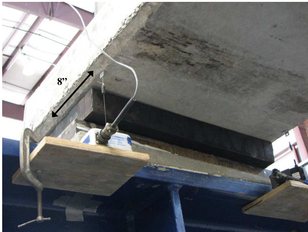
Figure F.1 – Bearing pad vertical displacement locations
