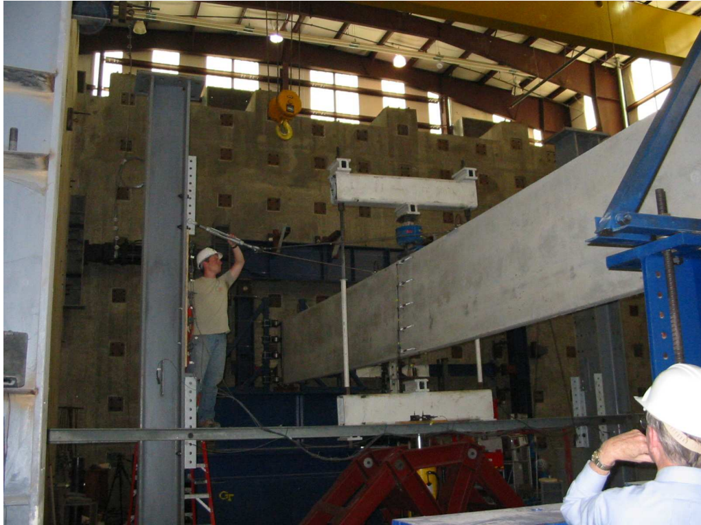
Figure 5.3 – Releasing restraint system during loading #1 of Beam B2A
