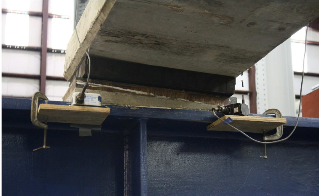
Figure 4.29 – String potentiometer layout at end supports beneath the girder
