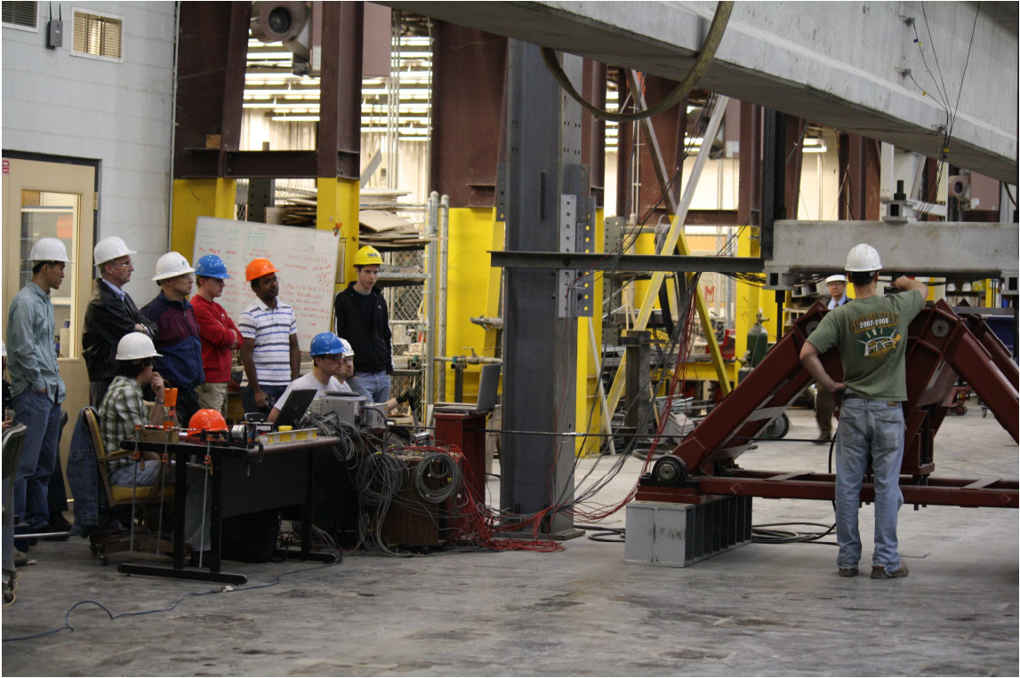
Figure 7.2 – BT-54 data acquisition and initial leveling
