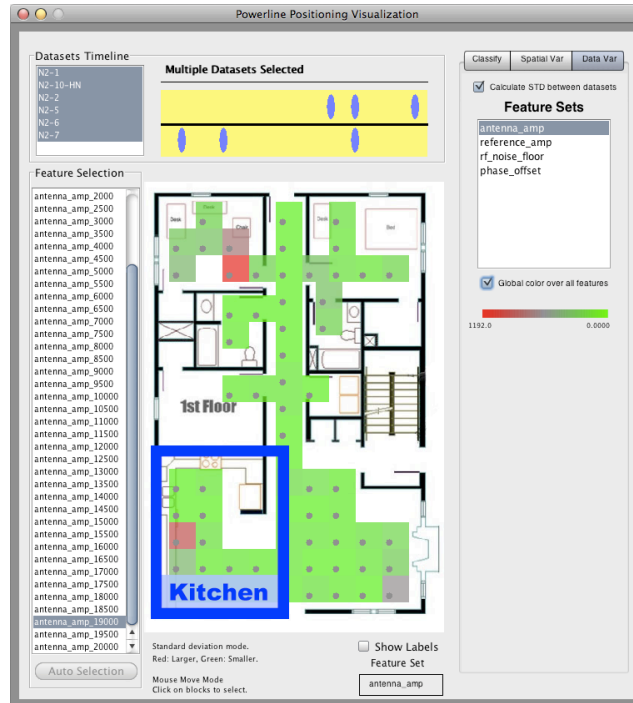
Figure 48: Standard deviation view of a selected feature in the Data Variance Perspective that shows several temporally unstable blocks. One is in the kitchen area and two are in the rooms at the back of the house.
