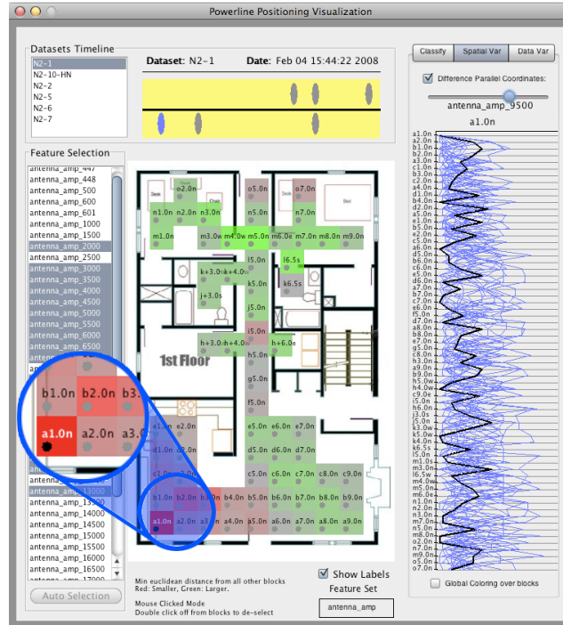
Figure 50: Selected block a1.0n is clearly closest to block b1.0n in the Spatial Variance Perspective.
