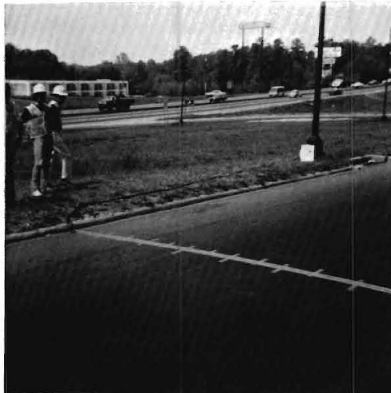
Figure 3. The road-tube installation, and its position relative to the camera. Gore area for this ramp is in background.
