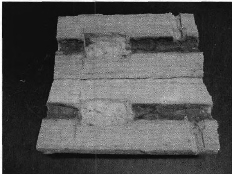
Figure 2.11: Photograph of the HEMJ divertor test section insulation.
