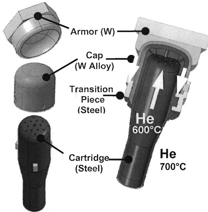
Figure 1.1: Diagram of the HEMJ divertor [4].
