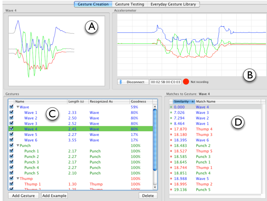
Figure 28: The Gesture Creation tab. A: recorded gesture view; B: live sensor view; C: list of gestures and gesture examples; D: sorted list of distances from currently selected example to every other example.
