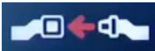
Figure 8: This airline “fasten seat belt” sign (from a Delta Airlines in-flight safety video) is an illustration of an annotated control diagram , showing stylized representations of the two parts to the seat belt, with an arrow indicating how they should be joined.
