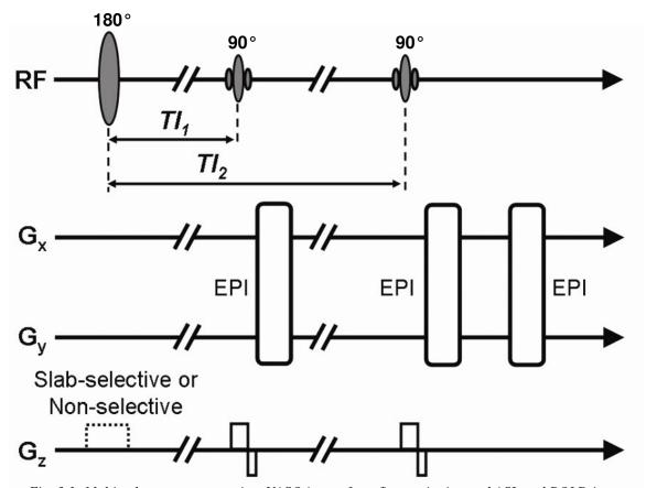
*Fig. 3.1: Multi-echo sequence acquires VASO image from first excitation and ASL and BOLD images from second excitation. (Sequence from Yang et al. [23])*
