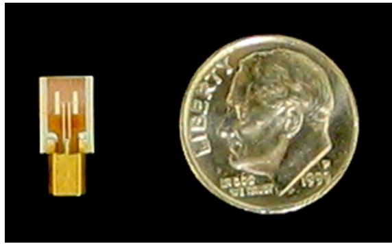
Figure 136. Photo of the singulated H-shaped antenna with the GPPO connectors.
