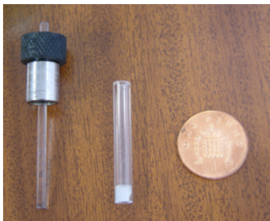
Figure 1.6: The quartz rod and capillary used for Couette flow with a 1p coin to give an idea of scale.
