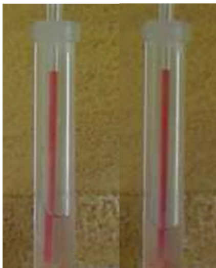
Figure 9.4: Photographs taken immediately after insertion of the inner capillary into the outer capillary (left) and after one hour. The inner capillary contains a red dye and the outer capillary water. The inner capillary is held at the same height as in the Couette flow cell.
