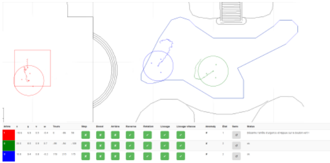
Fig. 10: User Interface screenshot, in production (9th of September, 10:30 to 10:45), where we can see the path recently taken by the AGVs, and a table with status and controls for each AGV.
