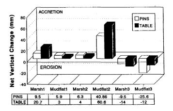
Figure 3: Sedimentation Pin and Table Net Change
