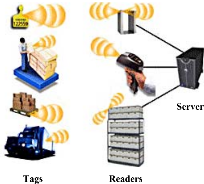
Figure 1.1: Conceptual diagram of an RFID system.
