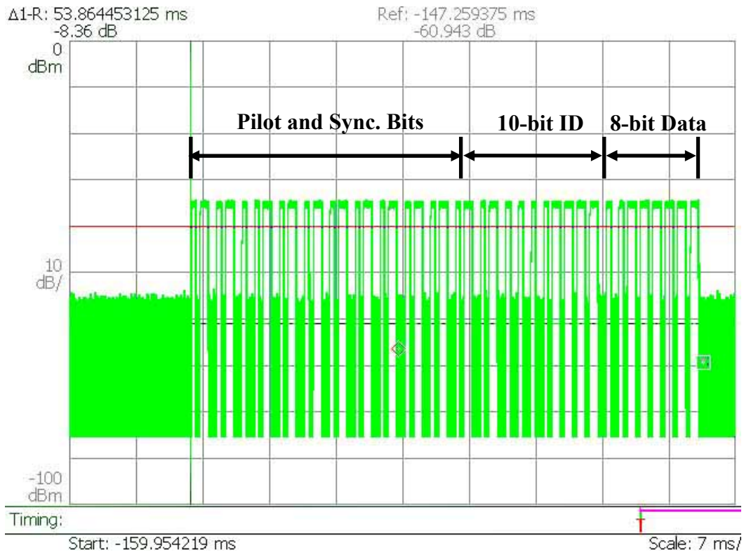
Figure 6.10: Diagram of the data sequence sent out by the active RFID tag.
