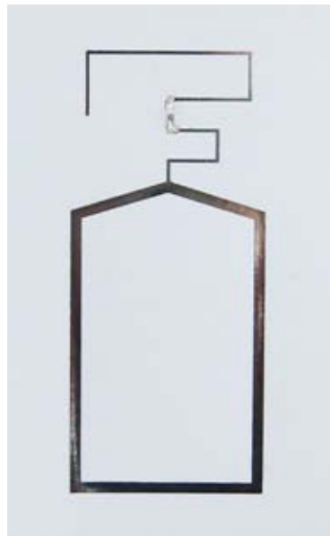
Figure 3.19: Photograph of the proposed inkjet-printed RFID tag on paper-based substrate with ink-usage optimization.
