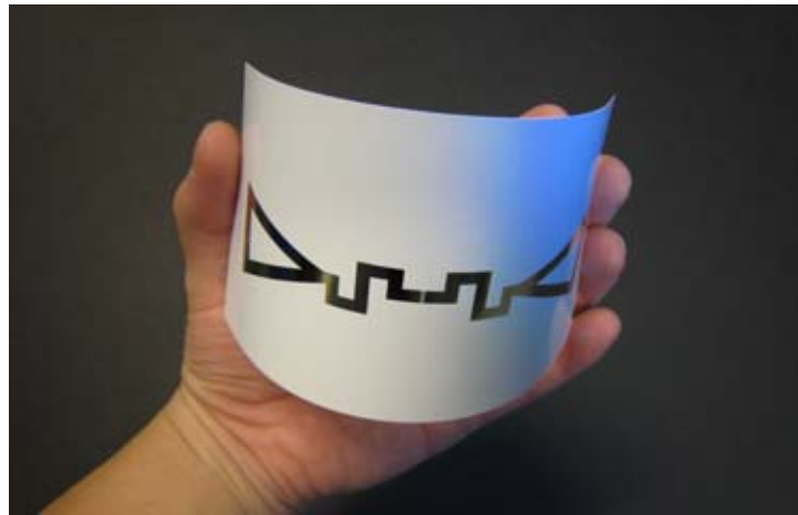
Figure 5.11: Photograph of the conformal tag with a SWNT film in the center.
