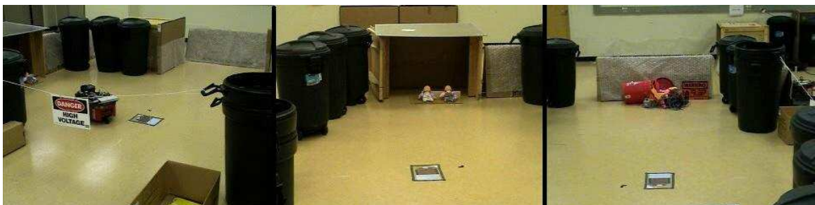
Figure 3.5 An overview of the maze environment used as a mockup of a simple search and rescue environment. One corner of the maze had two dolls representing children (center photo) and the other corner had a simulated fire and biohazard (right photo).
