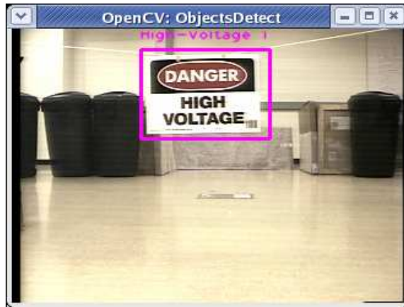
Figure 3.8 In laboratory experiments the robot uses landmark detection to aid navigation.
