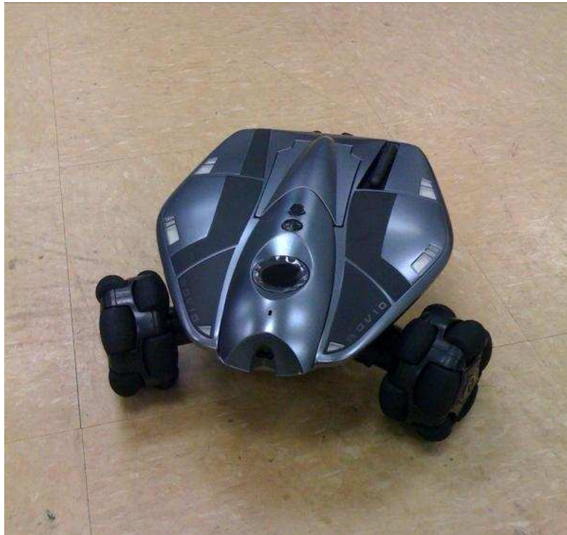
Figure 3.7 A photo of the Rovio mobile robot. The robot's neck is point towards the bottom of the image and is in the unextended position. The webcam is at the end of the neck.
