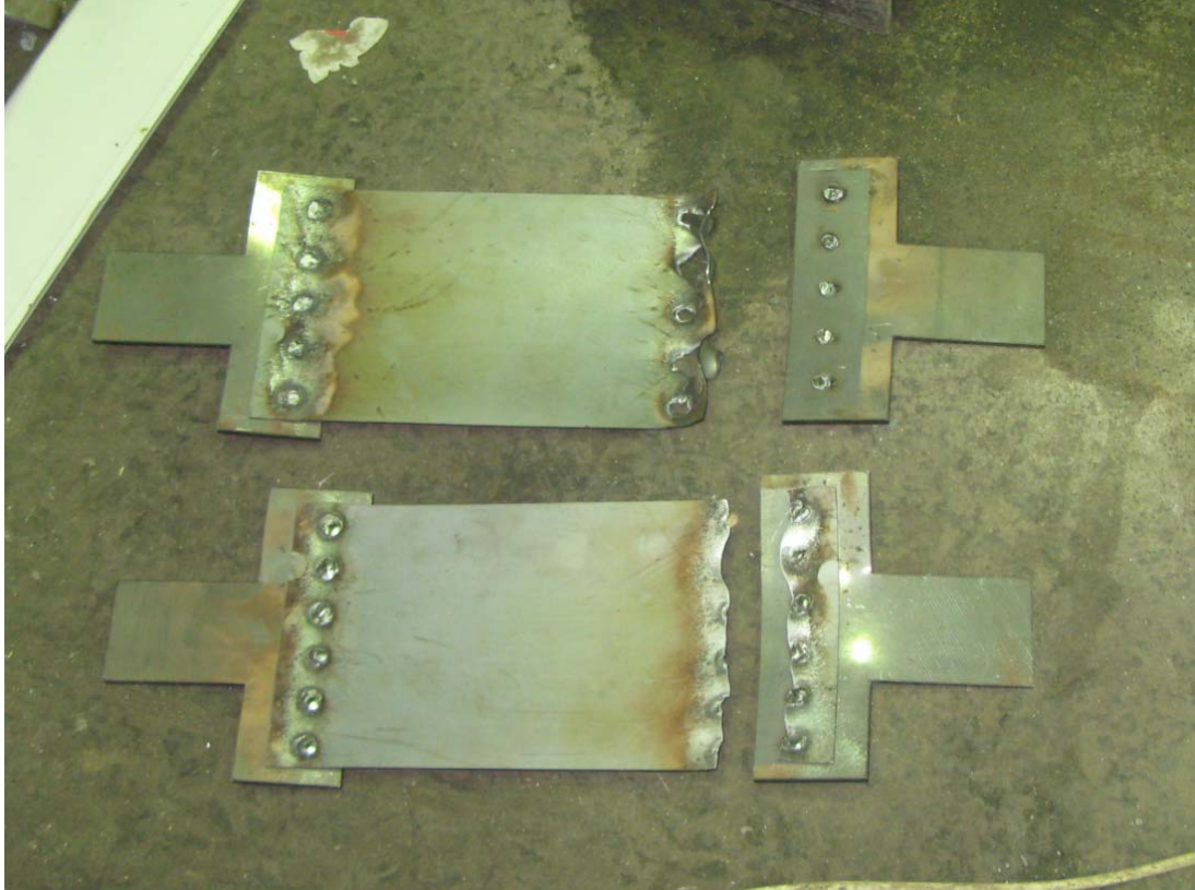
Figure 6.5: Failure modes; weld metal fracture (up) plate fracture (bottom)
