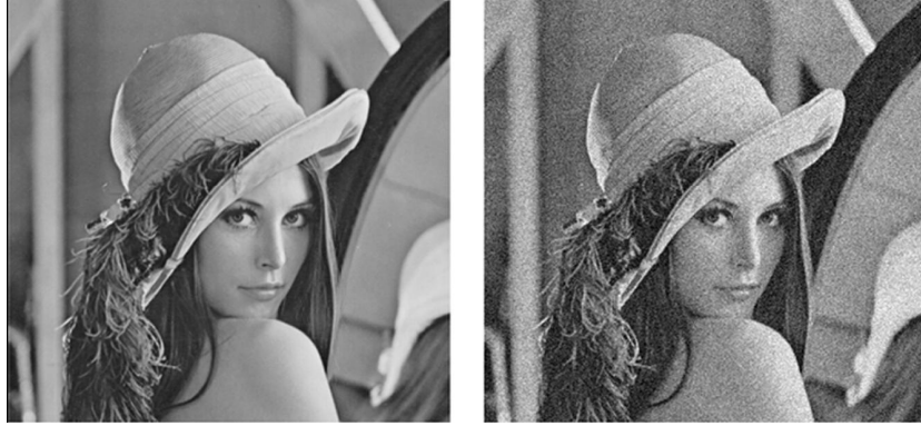
Figure 5: clean image (left); image with Gaussian noise, with standard deviation \sigma = 25 , SNR=5.64dB(right).
