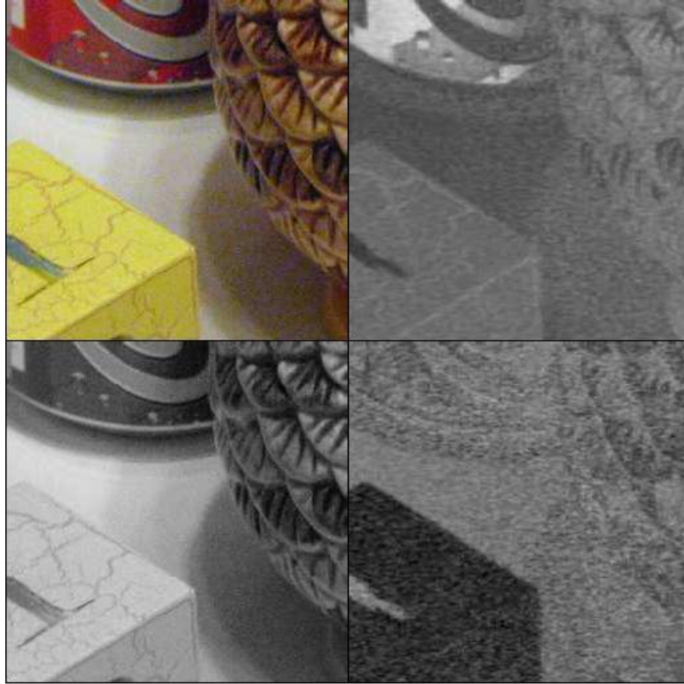
Figure 33: YCrCb Decomposition of an image with real noise. From left to right, top to bottom: original image, Cr channel, Y channel, Cb channel. Note that Y channel is clean.
