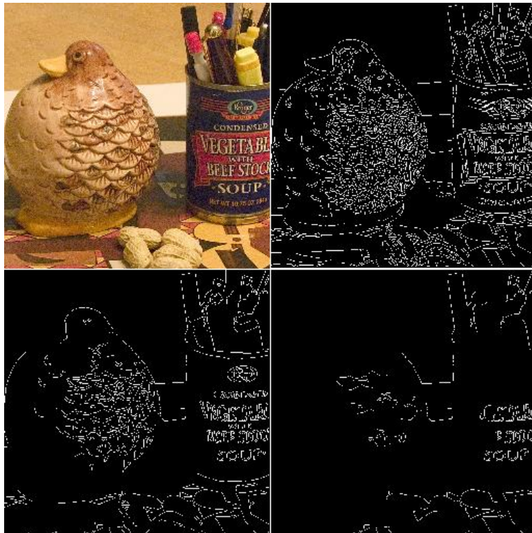
Figure 35: Canny's Edge Detection. Left top: original image with real noise; Right top: Canny's edge with threshold 0.15; Left bottom: Canny's edge with threshold 0.40; Right bottom: Canny's edge with threshold 0.15.
