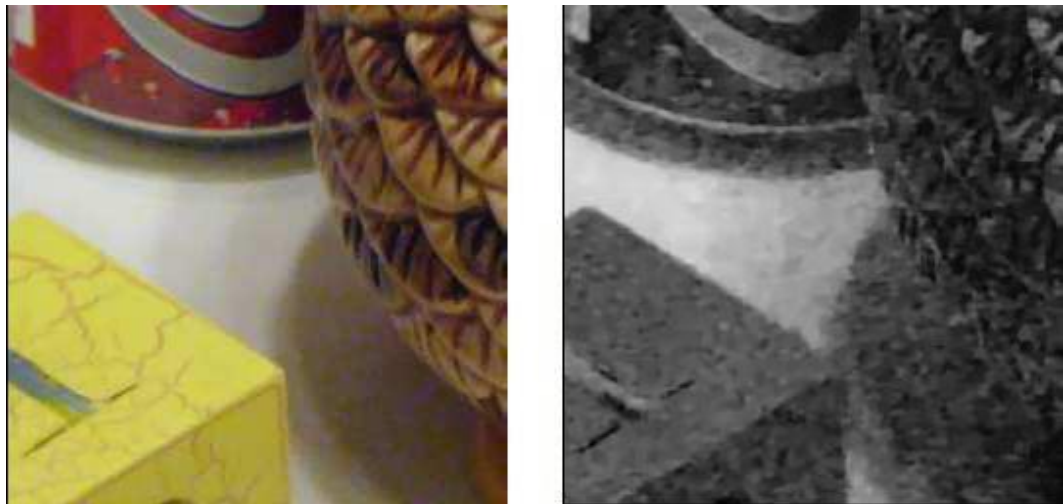
Figure 50: The denoised image by MTV in the RGB space (left) and its blue channel (right). Noticeable noise still exists due to high noise in blue channel even the recomposed image has most of the noise removed.
