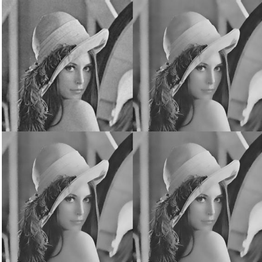
Figure 21: Lena image denoised by original bilateral filter with window size increasing. Left Top: 5 \times 5 , SNR=36.9857 , running time 16.953s; 20 \times 20 , SNR=32.587 , running time 37.484s; left bottom: 50 \times 50 , SNR = 32.2007 , running time 156.689s; right bottom: 100 \times 100 , SNR = 32.2007 , running time 591.001s.
