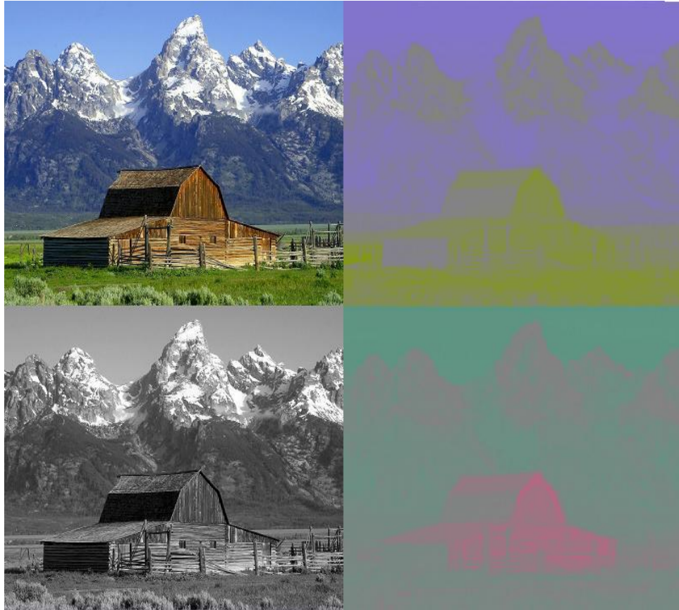
Figure 25: A color image(left top) and the Y(left bottom), Cb(right top) and Cr(right bottom) elements.
