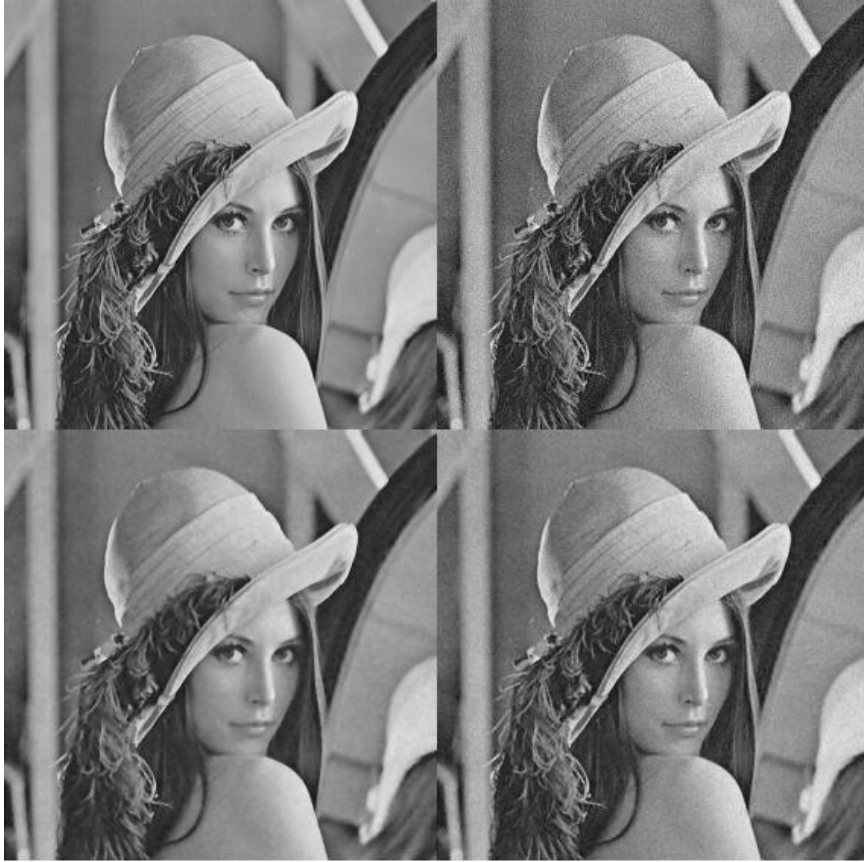
Figure 20: Left Top: original lena image; right top: lena with additive gaussian noise \sigma^2 = 25 ; left bottom: denoised by original non local mean filter, 1 iteration, SNR = 36.0472 ; right bottom: denoised by non local bilateral filter, 1 iteration, SNR = 37.1205 .
