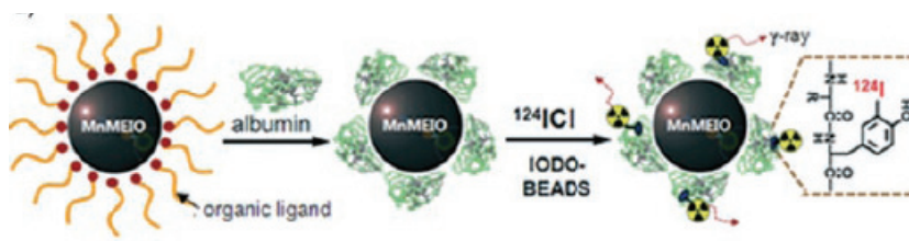
Figure 1.4: ^{124}\text{I} labeled, albumin coated \text{MnFe}_2\text{O}_4 dual PET/MRI nanoparticle (48).
