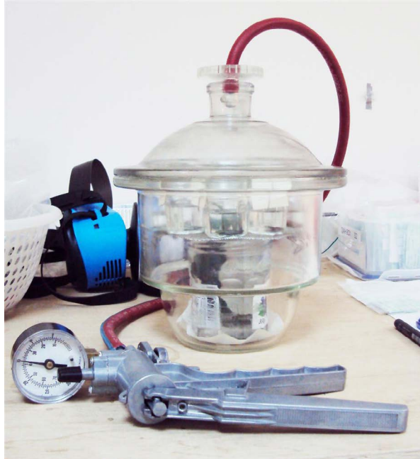
Figure 6.9: Lacquering the metals under vacuum
