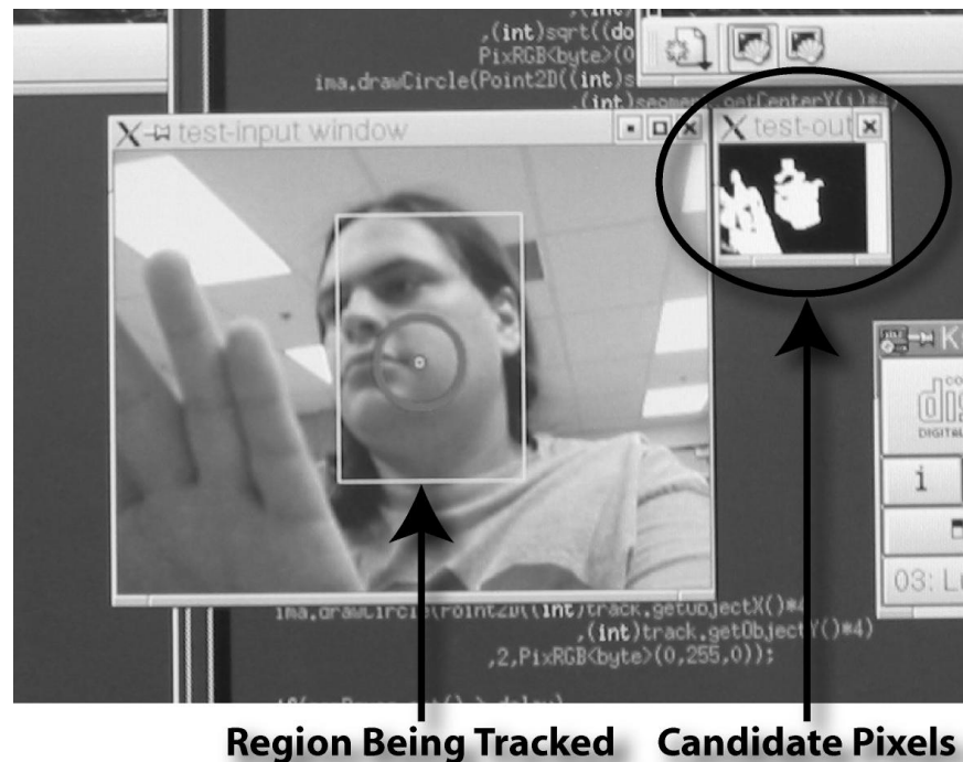
Figure 2: In this example the tracker is keying off of skin color along with the basic size ratios of the human head. Here it is quite adept at finding and tracking the human head even in the presence of a large number of distracters. Here it can be seen that the tracker is not fooled by the introduction of even the experimenters hand into the scene. This can be observed even though, in the candidate pixels window, the hand is a larger correct color target. Since the hand has slightly different color characteristics, even upon path crossing, the program still tends to follow the head due to adaptive color thresholding.
