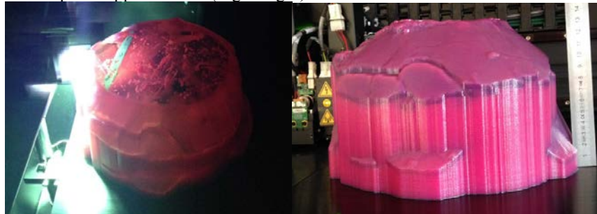
Fig. 6. Left: On-going 3D printing of the urn. Right: The printed urn with its support matter
